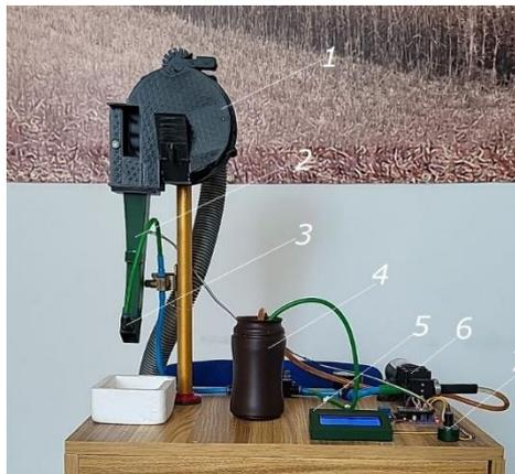
Figure 1. Model of pre-sowing seed inoculation system, where 1 - seeding device; 2 - sowing tube; 3 – nozzle; 4 - container for working fluid; 5 – monitor; 6 – water pump; 7 – encoder.
